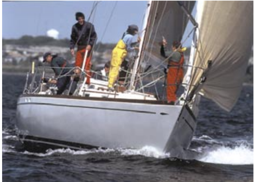
With her new all carbon fiber mast MISCHIEF, Sequin 40 built by Lyman-Morse in 1988, saved more than 110 lb. aloft and is noticeably faster on all points of sail.
